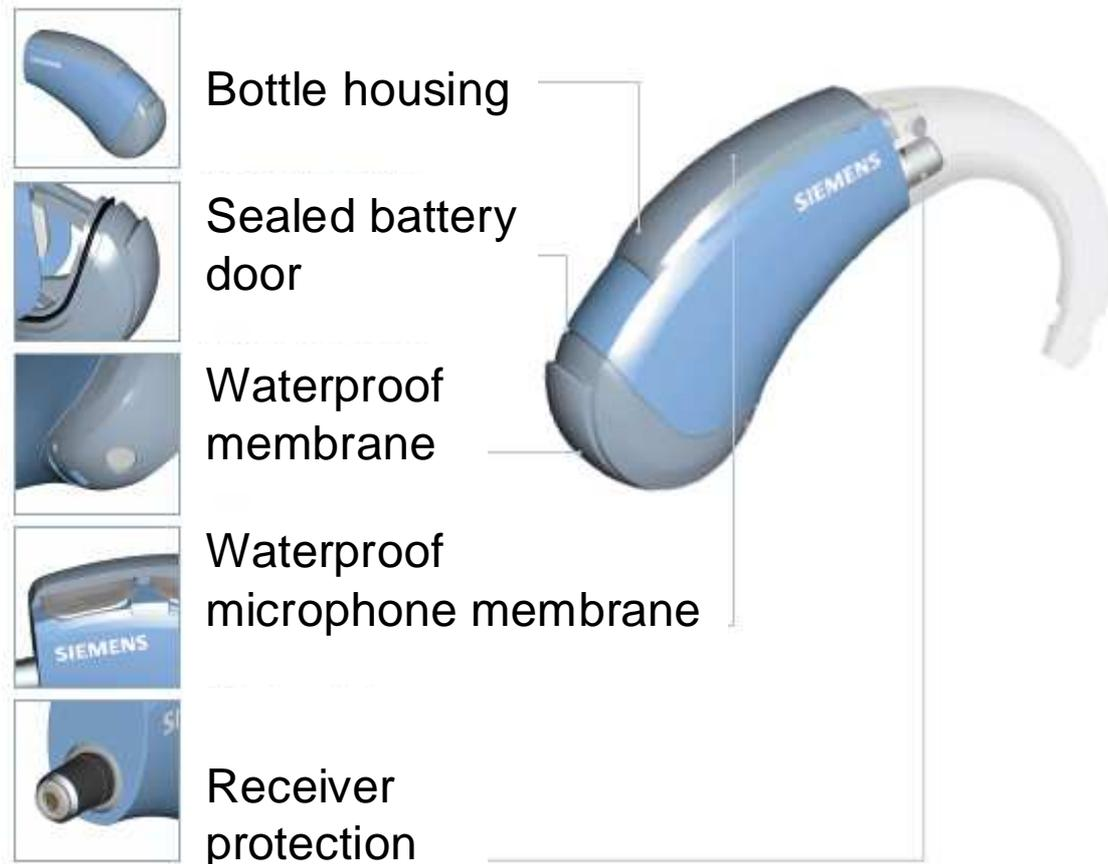
**Figure 1:** Illustration of five innovations to construct a properly functioning waterproof hearing aid
