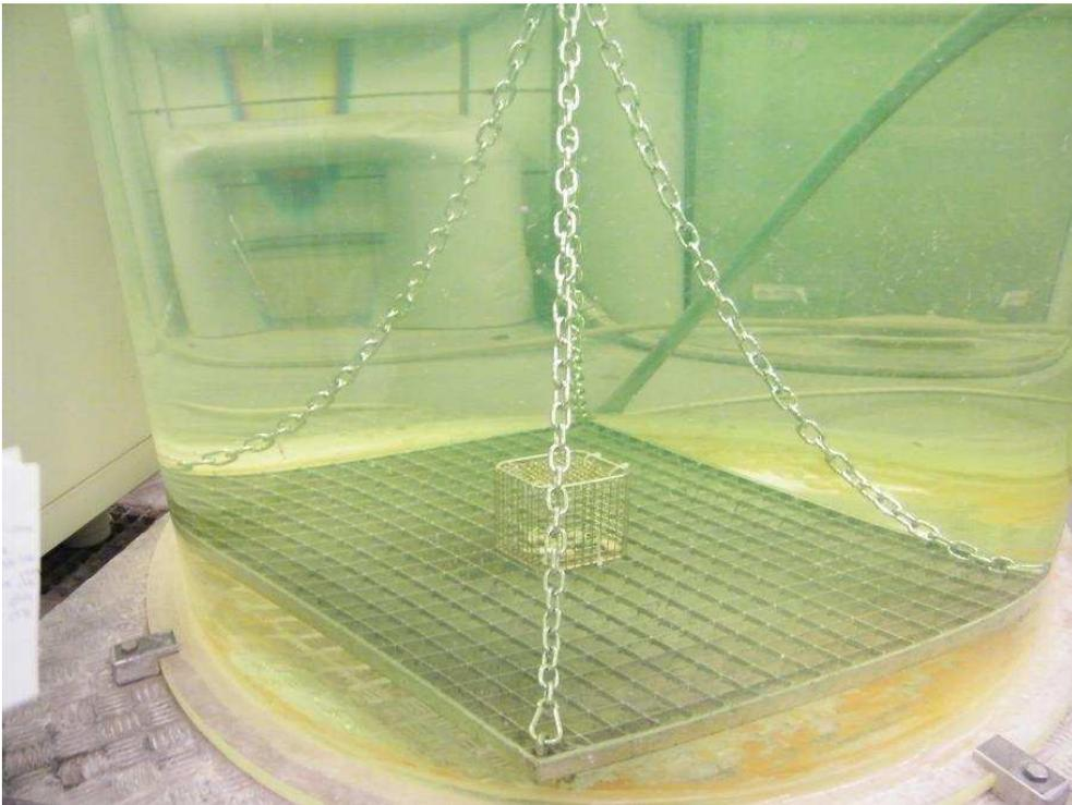
**Figure 3:** Test setup for IPX7, total submersion in water 1 meter deep for a duration of 30 minutes.
